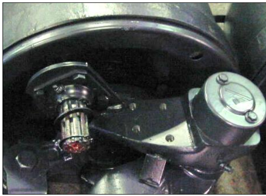
300 Series – ACB holes tapped directly into steer axle knuckle.
