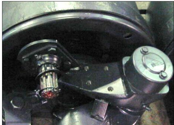
100 Series – ACB holes tapped directly into steer axle knuckle.
