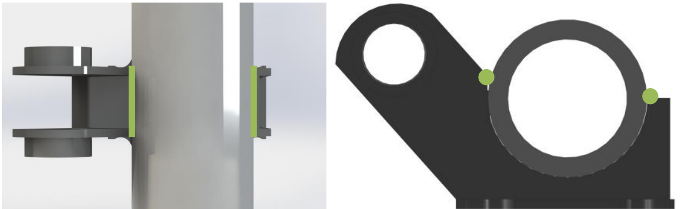
36146 Axle seat – Weld details
