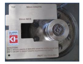
Is the Kingpin still squarely installed? Are there signs of damage to the kingpin? Are there any impact signs? Checked the mounting bolts? Will this kingpin last to the next check?
