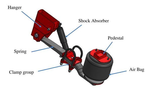
Hanger - This is the main connection of the suspension to the chassis. It supports the suspension spring and shock absorber. The hanger must be properly braced to the chassis to give the suspension the strength to withstand the forces on the suspension when cornering.
