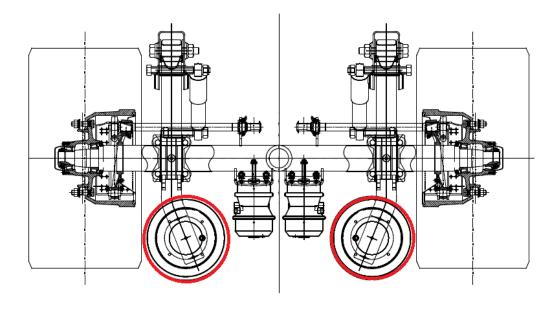
The air suspension air bag requires an air fitting and needs to be bolted to the vehicle chassis. If the vehicle has an enclosed box design a pedestal above the air bag would be needed to give space to secure the air bag mounting bolts and access for air fitting.
