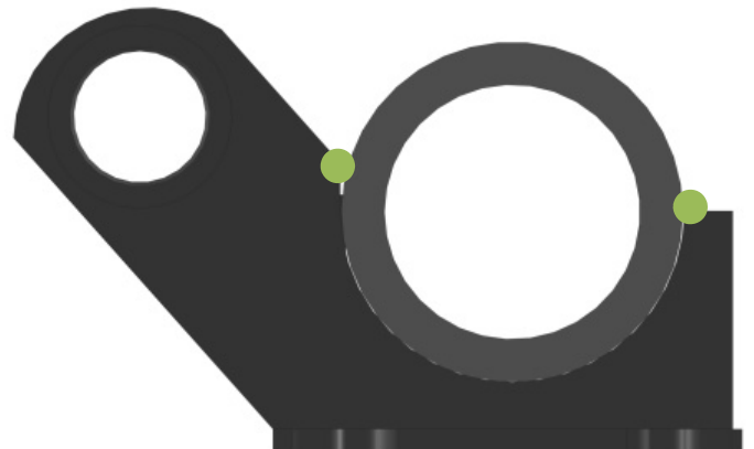
36146 Axle seat – Weld details
