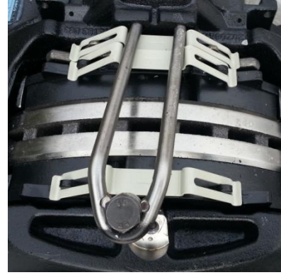
Lift away the retainer and bolt
