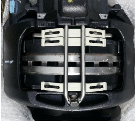
First gain access to the brake pads by removing the wheel. Loosen the retaining bolt.
